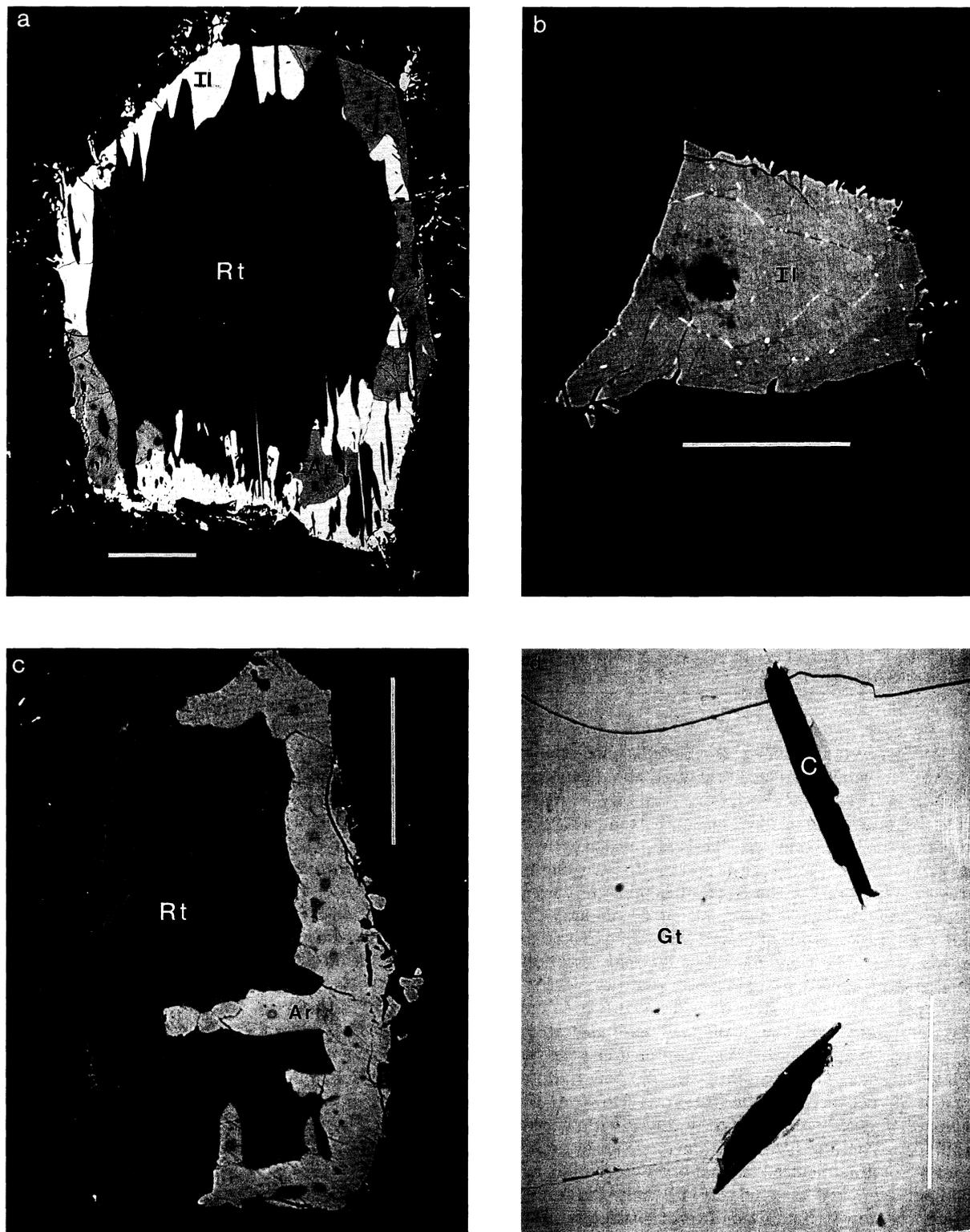
Fig. 3. Back-scattered electron (BSE) images of oxide textures. Scale bars are 50  $\mu\text{m}$ . (a) Rutile (dark) partially rimmed by armalcolite (medium) and ilmenite (bright) from sample ET11. (b) Ilmenite crystal from sample ET11; light and dark regions are ilmenite that contains varying amounts of Fe and Mg. (c) Rutile (dark) rimmed by armalcolite (bright) from sample ET42. (d) Primary graphite (dark) included in garnet from sample ET11.
