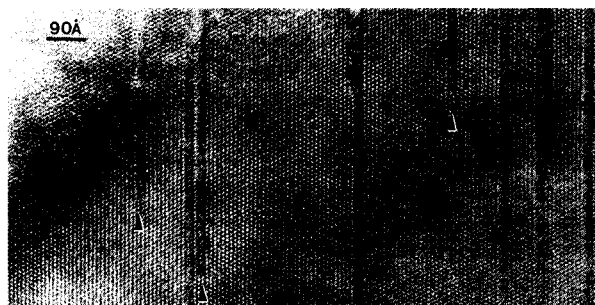
FIGURE 4. HRTEM image of tremolite quenched from 740 °C, showing (010) clinopyroxene slabs with thicknesses of 18 and 36 Å along the b axis. Arrows indicate terminations of clinopyroxene slabs.
