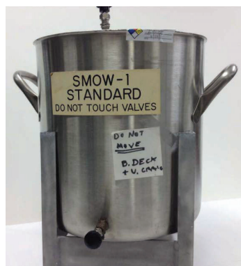
Figure 2. The SMOW-1 standard (VSMOW). Why, if it is not to be moved, does it have handles? [USGS Public Domain].
