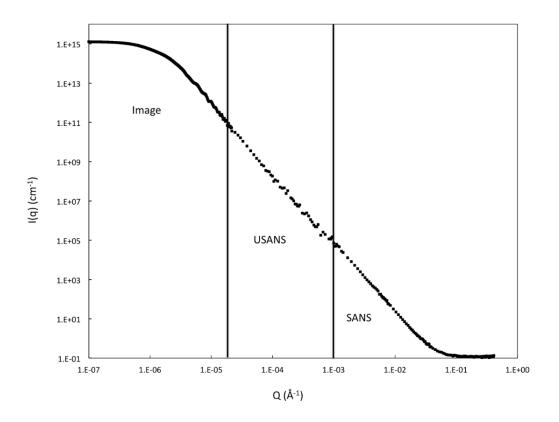
**Figure 32.** Example of radially integrated scattering data for a sandstone (sample 04Wi17b, 100°C, 8 weeks, Anovitz et al. 2015). The central part of the curve has a power-law slope of -3.538 ( $r^2 = 0.99925$ ). Ranges shown for data obtained from SEM/BSE imagery, USANS and SANS measurements are approximate as the data overlap.
