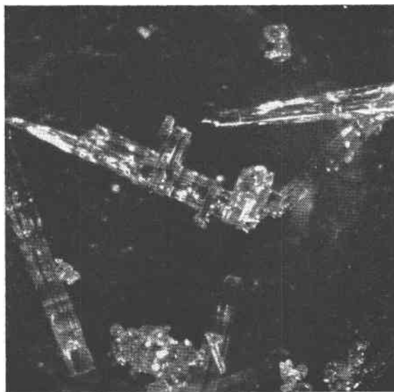
FIG. 7. Photomicrograph of wurtzite prism interrupted by layers or knobs of sphalerite ( \times 92 ).
