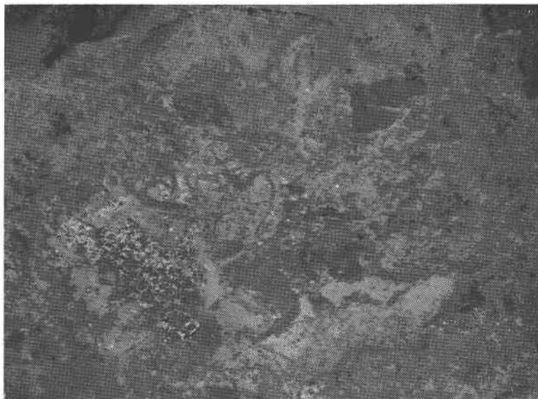
FIG. 1. Photomicrograph (ordinary light). The very bright small particles (lower left center) are hematite. The smooth fairly bright areas are jacobite; the brightness varies as it is oxidized and hydrated to limonite, which most of the darker areas represent. \times 45
