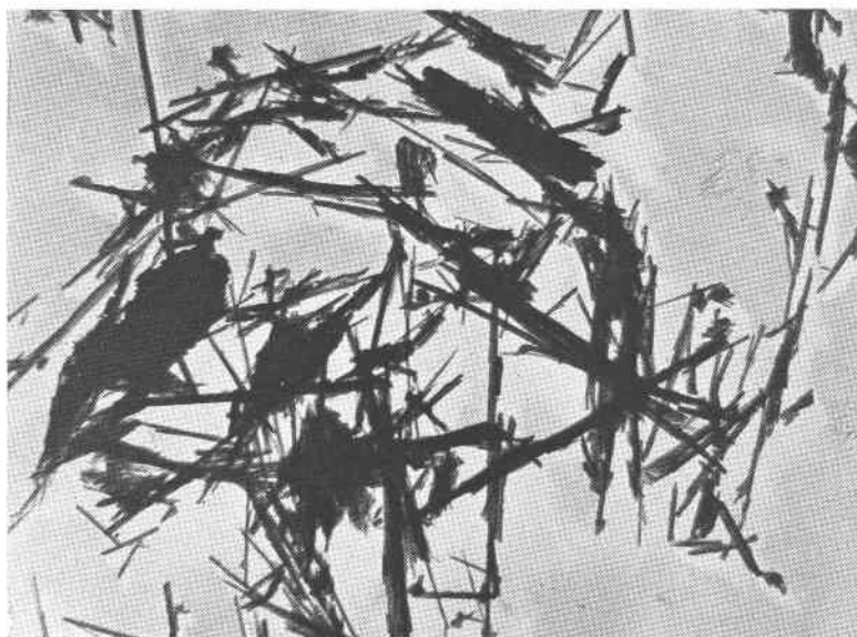
FIG. 2. Electron micrograph of povlen-type clinochrysotile; \times 8000 .
