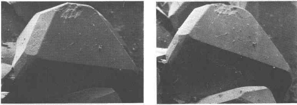
Fig. 5. Two scanning electron microscope photographs ( \times 100 ) of a crystal of calcite having an unusual habit. The photographs are related by a rotation of 23^\circ around an axis parallel to the bottom edge of the photographs.
