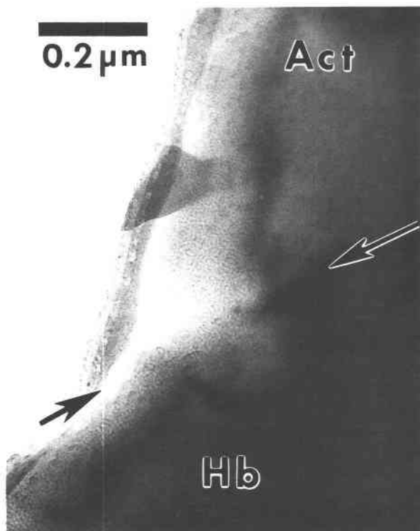
Fig. 4. Bright-field TEM image of thin edge of calcic amphibole inclusion shown in Fig. 1 (area 3, hollow arrow). The actinolite and hornblende are coherently intergrown. The grain boundary is at a low angle to the plane of the specimen and runs from lower left to upper right between the arrows. The electron beam is parallel to [012] of the amphibole.
