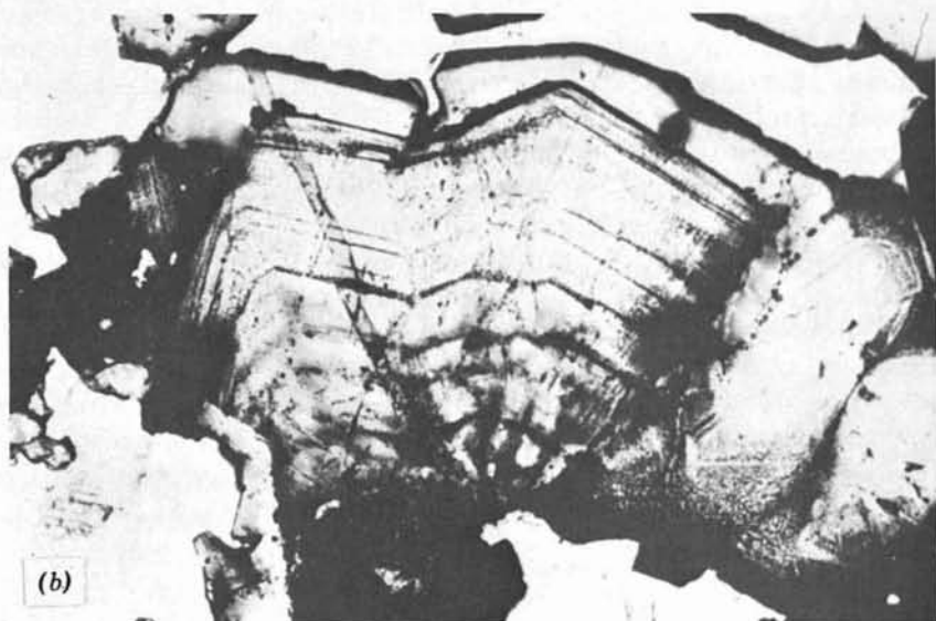
FIGURE 2.9 Comparison of the structure visible in the same sample of sphalerite when viewed: (a) in normal reflected light and (b) in transmitted light in a doubly polished thin section. (Figures courtesy of P. B. Barton, reproduced from Min. Geo. 28, 296, 1978, with the publisher's permission.)
