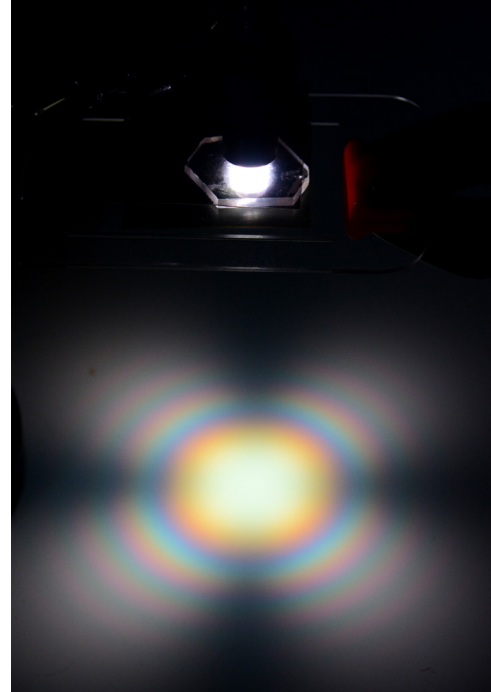
Figure 4: With the 3 mm basal slice of Figure 1 sandwiched between crossed polarizing filters, a fiberoptic light is used here to project the bull's eye optic figure onto a white surface.
